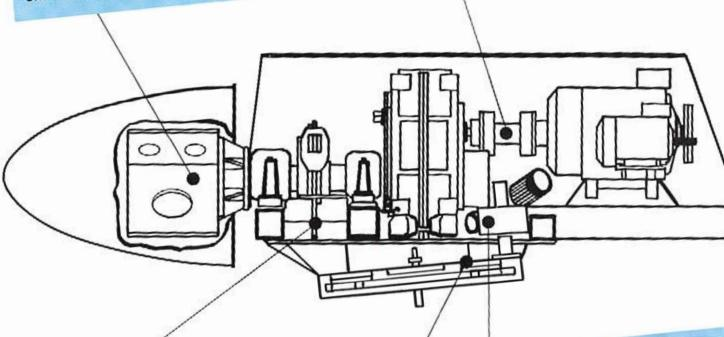
The windmill is equipped with an operation brake on the slowrevolving shaft. A fact which means that the gearbox will not be exposed to large mechanical loads when breaking.
